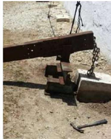
Some of the anchors previously installed by others were also tested and found to offer very little resistance to wind uplift, and pulled out of the ground with no additional load applied to the lever arm.
