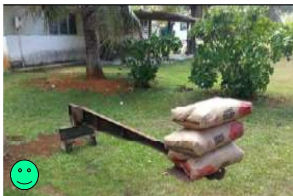
Anchors installed as part of the program are sampled and site-tested as part to the on-going quality control program, and provide excellent resistance to wind uplift. Cement bags are loaded onto a 10 : 1 lever system.
