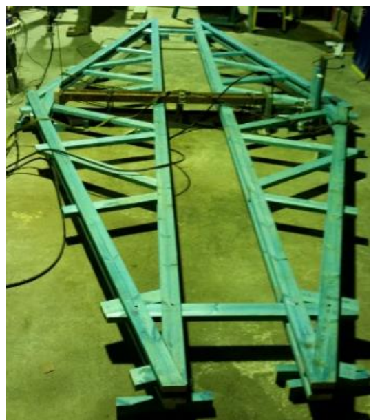
Two Test Trusses Being Pushed Apart
