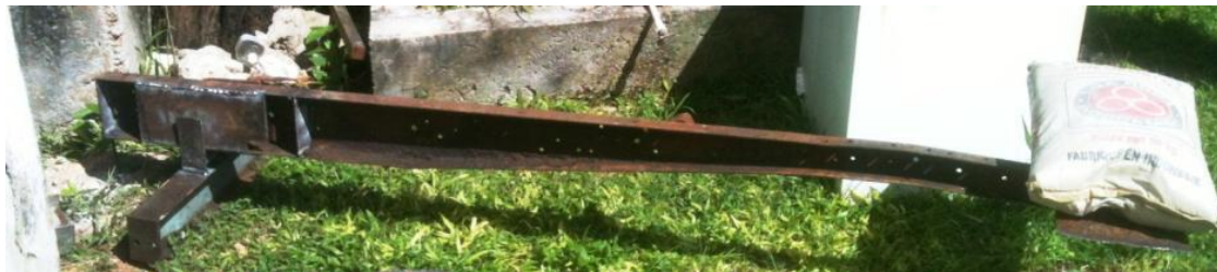
Prototype Proof Load Site Tester used in Mangaia, Cook Islands to test anchor bolts Copyright: Quasar Management Services Pty Ltd
