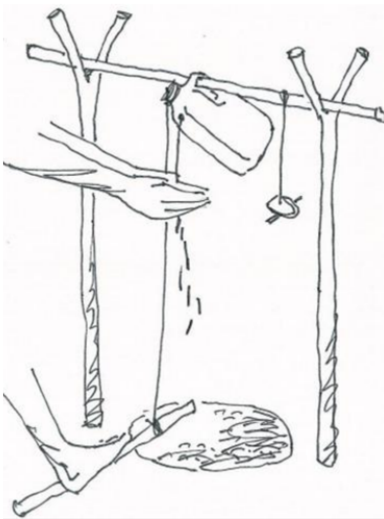
Figure A11: The Tippy Tap. (Acknowledgements regarding design and artwork: Emergency Architects Australia)
