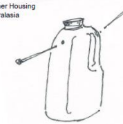
Heat the nail and make one water outlet hole and one air intake hole in the water container.
